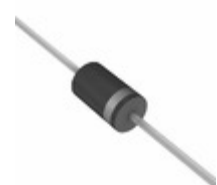
MUR460 R0G TSC (Taiwan Semiconductor) DIODE GEN PURP 600V 4A DO201AD
