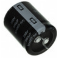
EET-UQ2S331JA Panasonic Electronic Components CAP ALUM 330UF 20% 420V SNAP
