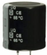
EET-UQ2S331DF Panasonic Electronic Components CAP ALUM 330UF 20% 420V SNAP
