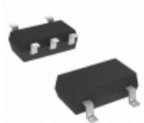
MIC5253-2.9BC5 TR Microchip Technology IC REG LDO 2.9V 0.1A SC70-5
