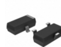
MMBT2222A Fairchild/ON Semiconductor TRANS NPN 40V 1A SOT-23
