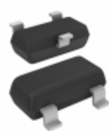
MMBT2222A,215 Nexperia USA Inc. TRANS NPN 40V 0.6A SOT23
