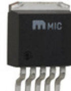
MIC39152WU Microchip Technology IC REG LDO ADJ 1.5A TO263-5
