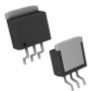
MIC39300-1.8BU TR Microchip Technology IC REG LDO 1.8V 3A TO263-3
