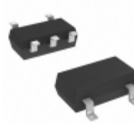
S-80133BNMC-JGST2U SII Semiconductor Corporation IC VOLT DETECTOR 3.3V SOT23-5
