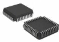
TS87C54X2-MCB Microchip Technology IC MCU 8BIT 16KB OTP 44PLCC
