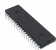
TS87C54X2-VCA Microchip Technology IC MCU 8BIT 16KB OTP 40PDIL
