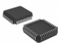
TS87C54X2-VCB Microchip Technology IC MCU 8BIT 16KB OTP 44PLCC
