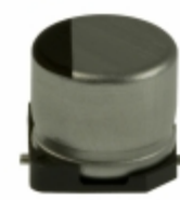
EEV-HA1C470P Panasonic Electronic Components CAP ALUM 47UF 20% 16V SMD
