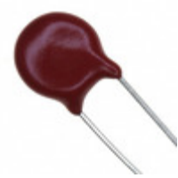
V150LU2 Littelfuse Inc. VARISTOR 240V 1.2KA DISC 7MM
