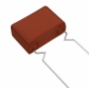
ECW-F2394HAQ Panasonic Electronic Components CAP FILM 0.39UF 3% 250VDC RADIAL
