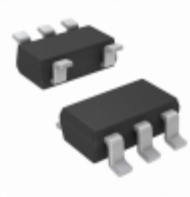
TC1186-2.85VCT713 Microchip Technology IC REG LDO 2.85V 0.15A SOT23-5
