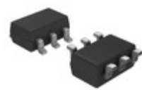
FDC645N_F095 AMI Semiconductor / ON Semiconductor MOSFET N-CH 30V 5.5A 6-SSOT
