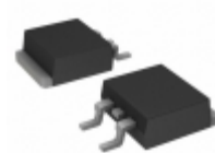
HUF75623S3ST AMI Semiconductor / ON Semiconductor MOSFET N-CH 100V 22A D2PAK
