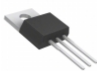
HUF75623P3 Fairchild/ON Semiconductor MOSFET N-CH 100V 22A TO-220AB
