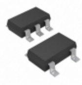
MIC94310-SYM5-T5 Microchip Technology IC REG LDO 3.3V 0.2A SOT23-5
