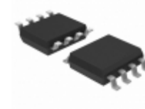
BR24T02FJ-WE2 Rohm Semiconductor IC EEPROM 2KBIT 400KHZ 8SOP- J
