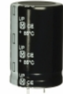
ECO-S1EP273DA Panasonic Electronic Components CAP ALUM 27000UF 20% 25V SNAP
