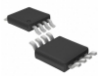
LTC1261LIMS8-4#TRPBF ADI (Analog Devices, Inc.) IC REG SWTCHD CAP INV -4V 8MSOP
