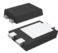
DXT2011P5-13 Diodes Incorporated TRANS NPN 100V 6A POWERDI5
