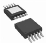
LT3042MPMSE#TRPBF ADI (Analog Devices, Inc.) IC REG LIN POS ADJ 200MA 10MSOP
