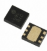
XC6122E621ER-G Torex Semiconductor Ltd IC WATCHDOG TIMER 6-USP
