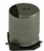
EEV-FC1H330P Panasonic Electronic Components CAP ALUM 33UF 20% 50V SMD
