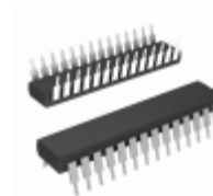
PIC16LC57C-04/SP Microchip Technology IC MCU 8BIT 3KB OTP 28SDIP
