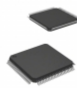
MB90F349CASPFV-GS Cypress Semiconductor Corp IC MCU 16BIT 256KB FLASH 100LQFP
