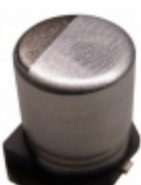
EMHJ100ADA331MHA0G Nippon Chemi-Con CAP ALUM 330UF 20% 10V SMD
