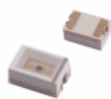
SML013WBD1 Rohm Semiconductor LED WHITE CLEAR 1208 SMD
