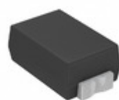
CDZT2R5.1B Rohm Semiconductor DIODE ZENER 5.1V 100MW VMN2
