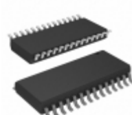
PIC16C72AT-20/SO Microchip Technology IC MCU 8BIT 3.5KB OTP 28SOIC
