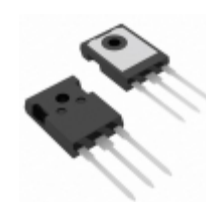
IXKH47N60C IXYS MOSFET N-CH 600V 47A TO-247
