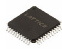
ISPLSI 1016E-80LTN44 Lattice Semiconductor Corporation IC CPLD 64MC 15NS 44TQFP
