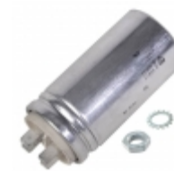
C870ZF35500AA0J KEMET CAP FILM 50 UF 5% 470 VAC MOTOR
