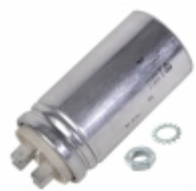
C878AF14400ZA4J KEMET CAP FILM 4UF 5% 500 VAC A2 MOTOR
