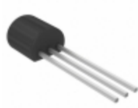
2N4403TA Fairchild/ON Semiconductor TRANS PNP 40V 0.6A TO-92
