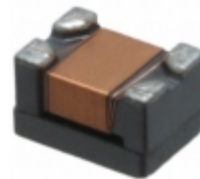
SRF4532-1R0Y Bourns Inc. CMC 1UH 1.2A 2LN 60 OHM SMD
