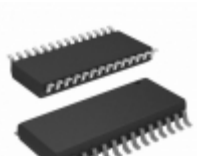
AT28HC256E-12SU-202 Microchip Technology IC EEPROM 256KBIT 120NS 28SOIC
