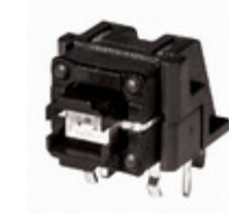
ITS40FR2ST C&K SWITCH TACTILE SPST-NO 0.05A 12V
