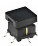
ITS23FV2SR C&K SWITCH TACTILE SPST-NO 0.05A 12V
