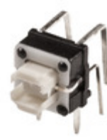
ITS40FR1ST C&K SWITCH TACTILE SPST-NO 0.05A 12V
