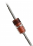
1N5241B AMI Semiconductor / ON Semiconductor DIODE ZENER 11V 500MW DO35
