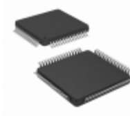
PIC24FJ64GA106T-I/PT Microchip Technology IC MCU 16BIT 64KB FLASH 64TQFP
