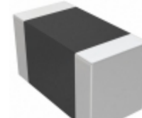
CC1206KKX7R8BB106 Yageo CAP CER 10UF 25V X7R 1206
