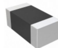
CC1206KKX7R8BB225 Yageo CAP CER 2.2UF 25V X7R 1206
