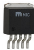
MIC5209-3.0BU TR Microchip Technology IC REG LDO 3V 0.5A TO263-5
