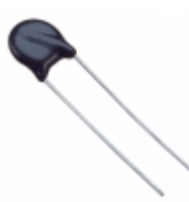
ERZ-V10D681 Panasonic Electronic Components VARISTOR 680V 3.5KA DISC 10MM
