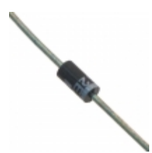
2EZ62D2/TR8 Microsemi Corporation DIODE ZENER 62V 2W DO204AL
