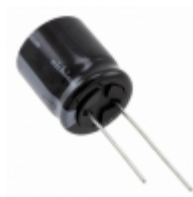
URS2D680MRD6 Nichicon CAP ALUM 68UF 20% 200V RADIAL
