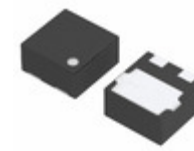
XC6120C162HR-G Torex Semiconductor Ltd IC SUPERVISOR 1.6V 3-USP
