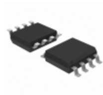
MCP6407-H/SNVAO Micrel / Microchip Technology IC OPAMP GP 1MHZ RRO 8SOIC
