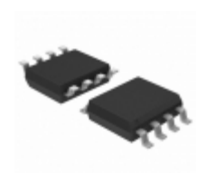
MCP6407-H/SN Microchip Technology IC OPAMP GP 1MHZ RRO 8SOIC
