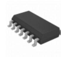
MCP6409T-H/SL Microchip Technology IC OPAMP GP 1MHZ RRO 14SOIC
