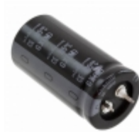
LGX2G391MELA50 Nichicon CAP ALUM 390UF 20% 400V SNAP
