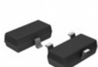
TC54VN2002ECB713 Microchip Technology IC VOLT DET 2.0V NCH OD SOT23A
