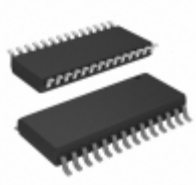
PIC18F2410-E/SO Microchip Technology IC MCU 8BIT 16KB FLASH 28SOIC
