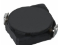
CDRH5D28NP-101NC Sumida America Components Inc. FIXED IND 100UH 420MA 520 MOHM
