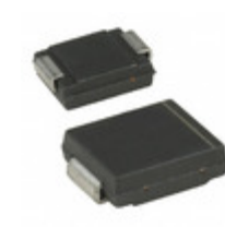
SM15T7V5AY STMicroelectronics TVS DIODE 6.4VWM 14.5VC SMC
