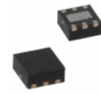
MIC5321-SLYMT-TR Microchip Technology IC REG LDO 3.3V/2.7V 0.15A 6TMLF
