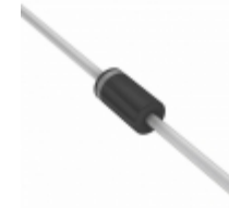
BZX85B56-TR Vishay Semiconductor Diodes Division DIODE ZENER 56V 1.3W DO41
