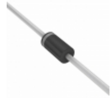
BZX85B56-TAP Vishay Semiconductor Diodes Division DIODE ZENER 56V 1.3W DO41
